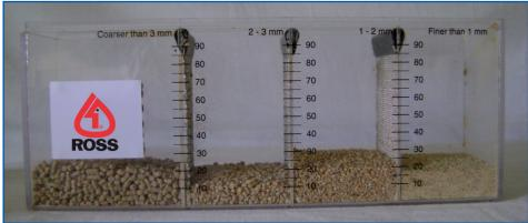
**Figure 4:** Sieving feed on farm before it enters the hopper to reduce percentage of fines presented to the birds.
